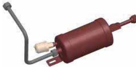
5. Remove the receiver dryer-condenser pipe and the pressure switch from the used receiver dryer and fit them to the new receiver dryer.
