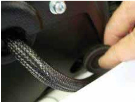
1. Remove the grommet at the bottom of the black evaporator casing
