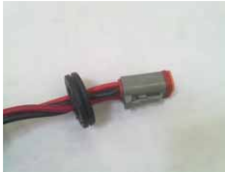
2. make a hole in the grommet and insert the cables through it.
