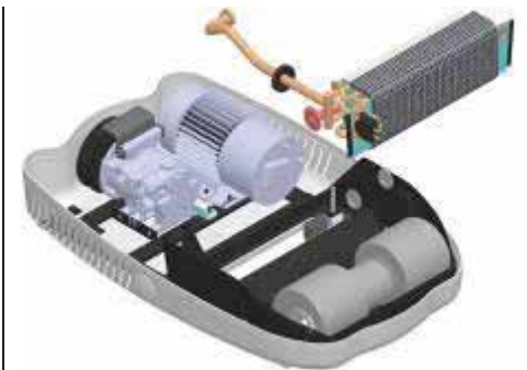
6. Lift the evaporator and change the evaporator foam. Put the evaporator back into place.
