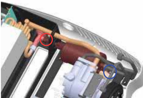
4. Take the receiver dryer fastening screw off (circled in blue), and disconnect the receiver drier connector on the expansion valve side (circled in red). Remove the compressor flange and the compressor-condenser pipe, and remove the receiver dryer.
