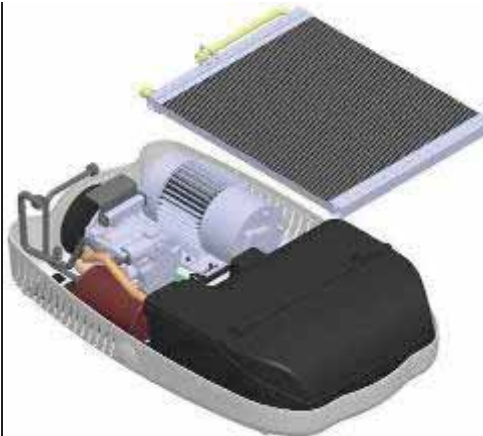
2. Remove the 4 condenser fastening screws, disconnect the 2 A/C pipes connected to the condenser, and remove the condenser.
