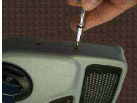
2. Plug the control panel connector back on, put the cabin panel back into place and fasten it with its 4 screws.
